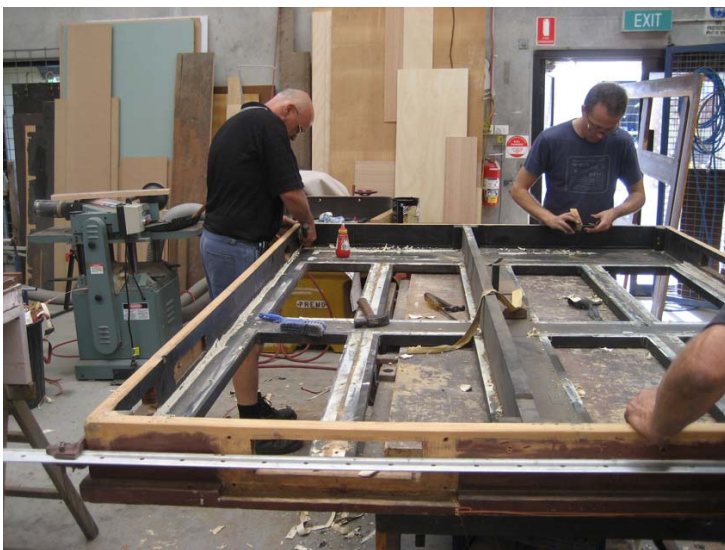
The bellows being repaired.
